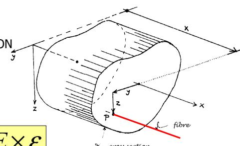
fibre in cross section  $x$  at position  $y, z$
