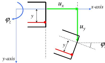
$$u(x, y, z) = u_x + z \times \varphi_y - y \times \varphi_z$$
