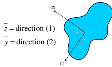
$$\begin{bmatrix} M_{\bar{y}} \\ M_{\bar{z}} \end{bmatrix} = \begin{bmatrix} EI_{yy} & 0 \\ 0 & EI_{zz} \end{bmatrix} \begin{bmatrix} K_{\bar{y}} \\ K_{\bar{z}} \end{bmatrix} \Leftrightarrow M_{\bar{y}} = EI_{yy} K_{\bar{y}} \quad M_{\bar{z}} = EI_{zz} K_{\bar{z}}$$
