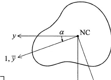
$$\begin{bmatrix} M_{\bar{y}} \\ M_{\bar{z}} \end{bmatrix} = \begin{bmatrix} EI_{\bar{y}\bar{y}} & 0 \\ 0 & EI_{\bar{z}\bar{z}} \end{bmatrix} \begin{bmatrix} \kappa_{\bar{y}} \\ \kappa_{\bar{z}} \end{bmatrix}$$
