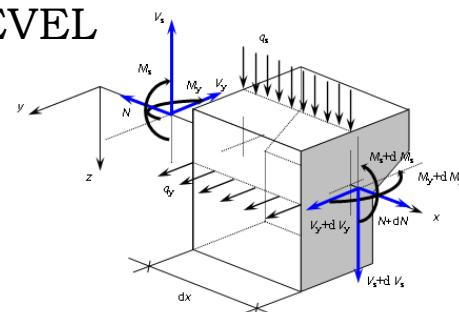
$$\frac{dN}{dx} + q_x = 0 \quad \Rightarrow \quad \frac{dN}{dx} = -q_x$$
