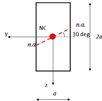
Determine the position of the plane loading  $m-m$  for the specified position of the neutral line which makes an angle of  $30^\circ$  degrees with the  $y$ -axis. The rectangular cross section is homogeneous.
